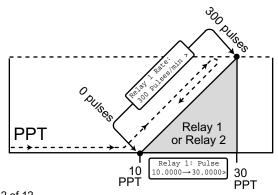
**Example 2:** As the process salinity (PPT) falls below the minimum pulse setpoint (30 PPT) the relay begins pulsing, triggering the metering pump for chemical addition. As the process salinity continues to decrease, pulsing accelerates proportionally until the maximum programmed pulse rate of 300 pulses/minute and setpoint (10 ppt) is reached, forcing the process salinity back up to intended levels (e.g.  $\leq$  30 PPT).
